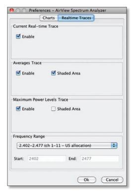
**Current Real-time Trace** When enabled, the real-time trace will be turned on. This is the yellow outline on the *Real-time* chart, which represents real-time power level of each frequency. The refresh speed depends on the FPS.
